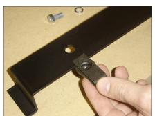
On each of the two custom brackets, install the Speed Nuts as shown.
