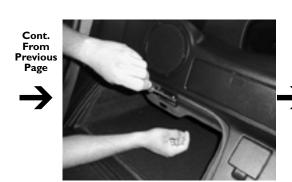
**STEP 15:** Remove the pair of Philip head screws securing the passenger side glove box's door latch.
