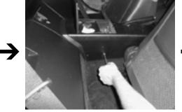
**STEP 4:** Remove the Philip head screws, that are found on both diver's side and passenger's side of the console.
