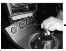
**STEP 8:** With the shifter trim panel moved to one side. Remove the pair of Philip head screws at the front edge of the console.
