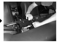
**STEP 14:** Remove the rear bulkhead front panel, by carefully pulling towards the front of the vehcile around the glove box.
