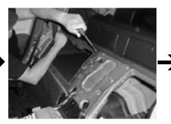
**STEP 17:** Remove the numerous 10mm head bolts securing the front edge of the glove box liner.
