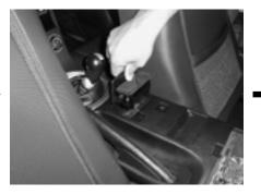
**STEP 5:** Remove the two Philip head screws that have been exposed by the removal of the ashtray.
