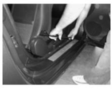
**STEP 3:** Remove the driver's side and passenger's side door sill panels.
