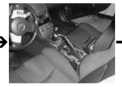
**STEP 13:** Remove the center console, out of the vehcile.
