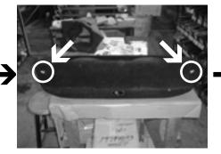
**STEP 21:** Thread in the supplied pair of socket cup set screws. Leaving about 1.5" exposed.
