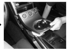
**STEP 6:** Loosen the shifter trim panel by pulling directly up. Pull the panel away from the console.
