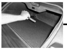
**STEP 16:** Remove the pair of 10mm head bolts at the rear of the glove box.
