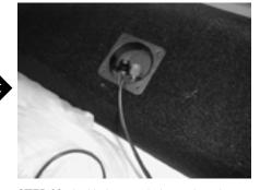
**STEP 22:** At this time, attach the speaker wire from the amp to the Stealthbox's terminal.
