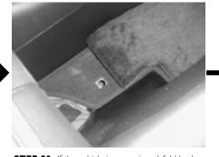
**STEP 20:** If the vehicle is so equipped, fold back floor mat as shown to access the mounting bolts.
