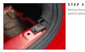
Remove the screw that holds the rear of the passenger side panel in place.
