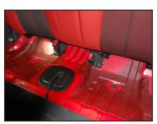
**STEP 8**Carefully unclip the front of the rear seat cushion, and remove the cushion.
