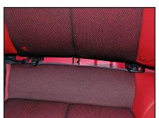
**STEP 7**Remove the bolts at the back of the rear seat cushion.
