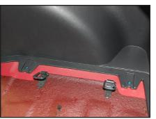
**S T E P 6**Remove the screws that hold the passenger side panel to the floor.
