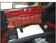
**STEP 4**Carefully unclip and remove the hatch sill panel.
