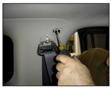
With a Phillip® screw driver, remove the screw that is located under the cover panel.
