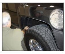
**STEP 22**Secure the driver's side rear plastic inner fender.
