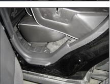
**STEP 5**At the driver's side rear door, remove the door sill.
