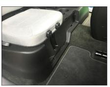
Remove the bracket from the storage tray. It will not be reinstalled.
