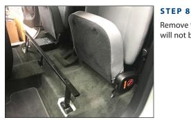
Remove the storage tray from the vehicle. It will not be reinstalled.
