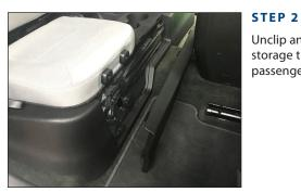
Unclip and remove the access panel from the storage tray below the rear seat on the passenger side. It will not be reinstalled.
