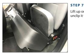
Lift up on the storage tray from the front to unclip it from the storage tray bracket.
