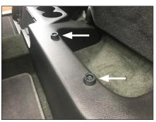
Remove the two screws and bumpers from the top of the storage tray on each side of the vehicle. They will not be reinstalled.
