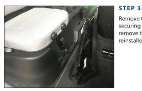
Remove the wing nut from the bracket securing the jack tools. Lift the bracket, and remove the tools. The wing nut will not be reinstalled.
