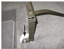
Remove the two Torx bolts and two nuts that secure the storage tray bracket to the vehicle.
