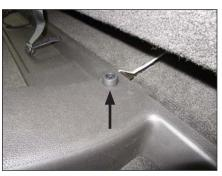
Remove the seven screws and bumpers from the top of the storage tray.
