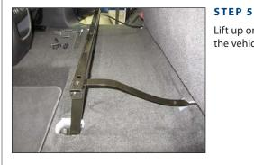
Lift up on the storage tray, and remove it from the vehicle. Pictured is the storage tray bracket.
