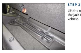
Lift the rear seat. Loosen the straps around the jack tools, and remove the tools from the vehicle.
