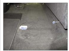
Remove the storage tray bracket from the vehicle.
