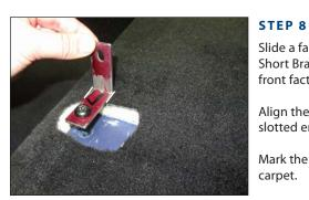
Slide a factory Torx bolt through the hole in a Short Bracket, and partially thread it into the front factory hole.
