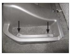
**STEP 3**Loosen the two clips from each side of the under-seat storage tray.
