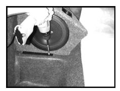
**STEP 4:** Using the supplied four self-tapping screws. Seucre the enclosure's moutning bracket to the flooring of the vehcile.
