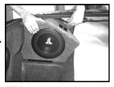
**STEP 3:** Insert the enclosure into the cubbyhole, taking care to loft and tuck the wiring harness above the enclosure as you slide as you slide it in. Push the enclosure firmly into place
