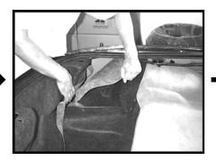
**STEP 2:** Remove the driver's side carpet from the cubby-hole in the corner of the hatch. this piece of carpet will not be used in the installation. Vehicle owner should keep this carpet for possible future use, when removing the Stealthbox.
