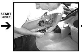
**STEP I:** Remove the driver's side trim panel, disconnect the speaker wires, if applicable.
