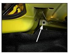
Locate the indicated hole. Slide a 3/8" Fender Washer over the 3/8 - 16 x 1-1/2" Hex Bolt, and insert it through the hole from the back side.
