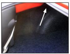
**STEP 1**Empty the trunk of the vehicle. The hardware installation area is indicated
