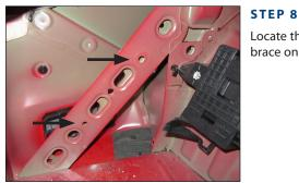
Locate the two indicated holes in the factory brace on the driver's side.
