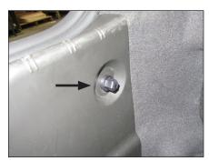
Remove the trunk floor panel from the vehicle. Unscrew the four clips from the rear sill panel, and remove the panel from the vehicle.
