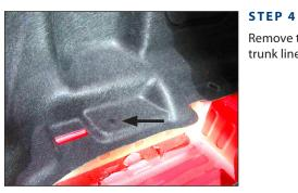
Remove the lower clip from the driver's side trunk liner panel.
