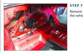
Remove the driver's side trunk liner panel from the vehicle.
