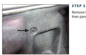
Remove the upper clip from driver's side trunk liner panel.
