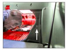
Remove the front clip from the driver's side trunk liner panel.
