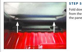
Fold down the rear seat, remove the two clips from the center trunk liner panel, and remove the panel from the vehicle.
