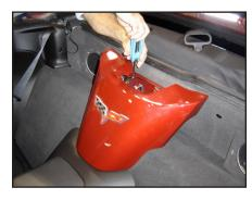
**S T E P 3** Remove the pair of Allen head screws from the top side of the painted interior trim piece.
