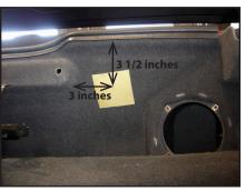
**STEP 5** Place a supplied wax squares onto the driver's side of the rear bulkhead.
