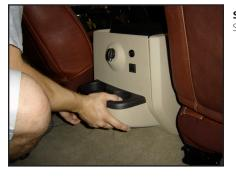
**S T E P 3 5**Secure the rear panel of the factory console, from **STEP 4**.
