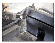
**STEP 13**With an air saw or similar tool, cut out the marked section.
