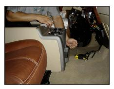
**STEP 3 4**Secure the front panel of the factory console, from **STEP 3**.
