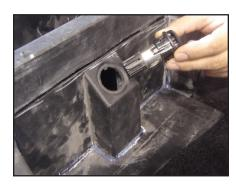
**S T E P 11**Remove the 12v plug from the inner area of the storage console.
