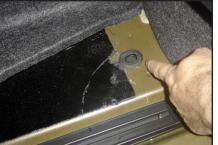
Remove the rubber body grommet towards the back of the floor as indicated.
