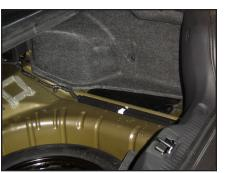
**STEP 2**Remove the trunk floor covering.
