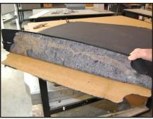
Peel back a section of the carpet from the top of the trunk floor panel as shown.
