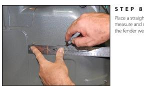
Place a straight edge under the protruding stud, and measure and mark 5-1/2" over from the vertical feature on the fender well as shown.
