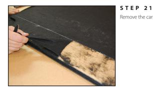
Remove the carpet from the back of the trunk floor panel.
