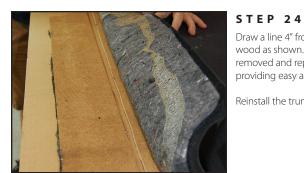
Draw a line 4" from the edge, and cut off the section of wood as shown. This will allow the trunk floor panel to be removed and replaced without removing the Stealthbox\*, providing easy access to the spare tire.
