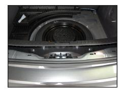
**STEP 5**Carefully unclip the rear sill panel, and remove the panel.
