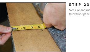
Measure and mark 4" from the passenger's side edge of the trunk floor panel.  $\,$
