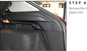
Remove the two Torx screws from the passenger's side plastic trim.
