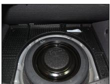
**STEP 4**Remove the trunk floor panel.
