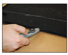
Cut the carpet around the edge of the trunk floor panel so that this section of carpet can be separated from the trunk floor panel.
