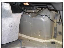
Pull the trunk liner and padding down and out from under the plastic trim as shown.
