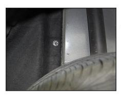
**STEP 1**Using a panel tool, remove the two star nuts from the inner fender panel of the passenger's side rear tire well.
