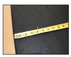
**STEP 17**On the under side of the trunk floor panel, measure and mark 4" from the passenger's side edge.
