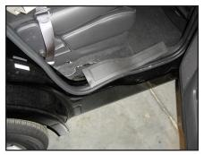
**STEP 2**Remove the passengers side rear door sill.
