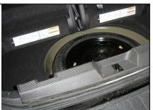
Remove the false floor and, the tailgate, and door sill.
