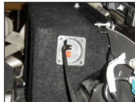
STEP 27 Run speaker wire from the amplifier location to the Stealthbox® location.
