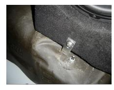
**S T E P 1 6**Using a 1/4"-20 x 1 Bolt, a 1/4" Lock Washer, and a 1/4" Flat Washer, attach the Large Bracket to the Stealthbox®, and hand tighten.
