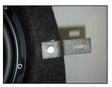
**S T E P 1 2**Attach the Z-Bracket to the front of the Stealthbox® using a 1/4"-20 x 1 Bolt, a 1/4" Lock Washer, and a 1/4" Flat Washer, as shown, and hand tighten.
