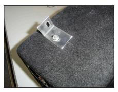
**S T E P 1 3**Attach the L- Bracket to the top of the Stealthbox® using a 1/4"-20 x 1 Bolt, a 1/4" Lock Washer, and a 1/4" Flat Washer, as shown, and hand tighten.
