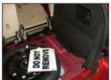
Remove foam filler panel or plastic storage tray from passenger side of spare tire.
