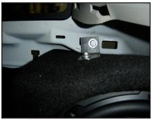
**STEP 17**Using a 1/4"-20 x 1 Bolt, a 1/4" Lock Washer, and a 1/4" Flat Washer, attach the L- Bracket to the Stealthbox®, and hand tighten.
