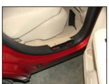
**STEP 5**Remove passenger side threshold plate.
