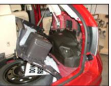
Remove passenger side cargo panel by prying away from side of vehicle and floor. If equipped, unbolt and remove the factory subwoofer enclosure.
