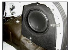
**STEP 19**Pictured is the Stealthbox® secured into position.
