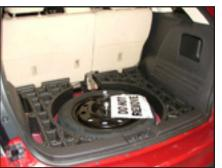
**STEP 1**Remove the floor panel by lifting seat flaps. Carefully tilt entire panel to exit hatch diagonally.
