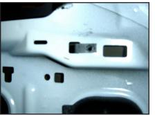
**STEP 9**Insert a 1/4"-20 U-Nut into the square hole near the side window, as shown.
