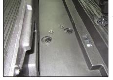
Remove the two factory nuts from each side of the tray.
