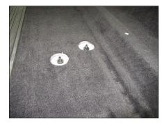
Reinstall the factory nuts on the studs, and fully tighten.
