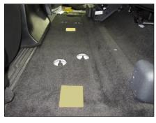
Carefully remove the Stealthbox<sup>®</sup> from the vehicle without moving the two Wax Squares.
