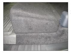
Align the Trim Panel with the driver's side of the enclosure, as shown.
