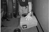
STEP 4: Place the Stealthbox into the passenger's side cavity and push down.
