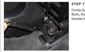
Firmly tighten the two 3/8 - 16 x 1-1/4" Hex Bolts, then firmly tighten the two factory seat bracket bolts.
