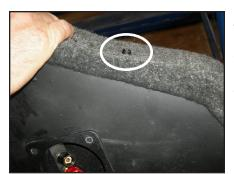
Thread the included 3/8-16 x 2 1/4" Allen Head Set Screw into the enclosure with the Allen socket facing out and approximately 1/4" exposed as shown.
