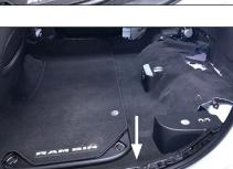
**STEP 12** Carefully unclip and remove the driver's side rear door sill panel.
