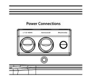
The JD400/4's **\*+12 VDC" and "Ground"** connections are designed to accept 4 AWG power wire. **4 AWG copper wire is a minimum power** wire size for this amplifier.
