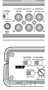
If you wish to send four discrete channels into the JD400/4, simply use all four inputs and set the "**Input Mode**" switch in the "**4 Ch**." position.
