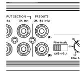
**Note:** The preamp output signal is not affected by the amplifier's filter controls. If the input signal is full-range, the preamp output will be full-range.
