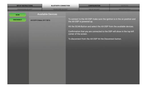
• **Scan** - Press this button to start the Bluetooth pairing process, then select the interface once it is found. "Connected" will appear in the top left corner of the app once paired.
