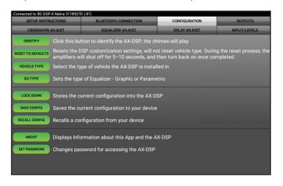
**RESET TO DEFAULTS**: Resets the interface to factory settings. During the reset process the amplifiers will shut off for 5-10 seconds.
