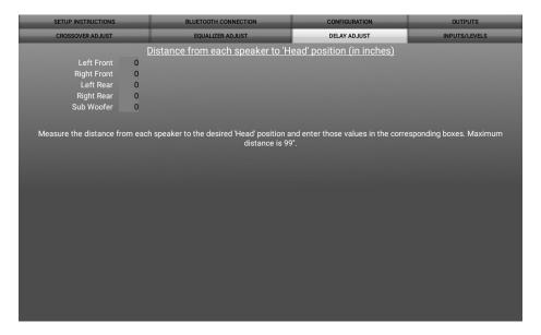
• Allows a delay of each channel. If a delay is desired, first measure the distance (in inches) from each speaker to the listening position, then enter those values to the corresponding speaker. Add (in inches) to the desired speaker to delay it.
