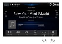
① Displays up to 15 labels obtained from iDataLink. A generic list, popup window, or current source screen is displayed by touching the Custom1 to 15 buttons. The screen that is displayed is determined by iDataLink.
