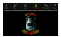
If the car sensor detects an obstacle, the screen automatically changes to the Parking sensor screen. For details, see "About Parking Sensor screen" (page 75).
