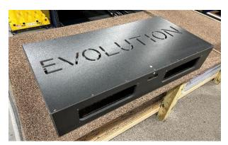
12. With the first four panels secure, add the top as shown, which is marked as Panel #5.
