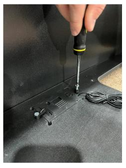
14. Secure the temperature and humidity gauge in place by using the screws and plastic clips as shown.
