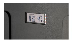
NOTE: The temperature and humidity gauge will record your minimum and maximum temperatures and humidity levels. This is a valuable tool to check from time to time to ensure that your enclosure is maintaining correct temperature and humidity fluctuations.
