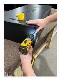
13. Add the final panel, marked Panel #6. This panel is the rear of the hood. Make sure it is positioned as shown. As in previous steps, please make sure that the first corner is correctly aligned before inserting the screws around all four sides.
