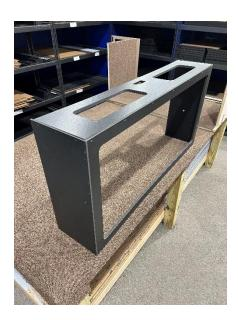
11. Carefully add the rest of the screws to fasten Panel #4, screwing in the ends securely. Be mindful as you go, in order to maintain a flush alignment of the panel edges.
