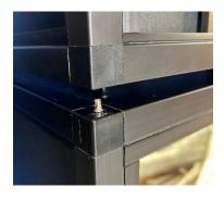
4. Now you can add the  $\frac{1}{2}$ " Lower/Bottom template stickers to the corresponding plastic corners on the bottom of the unit that will sit onto the steel pins. Drill out the holes with the larger  $\frac{1}{2}$ " drill bit so that this part will now sit over the steel pin as shown.
