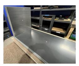
1. Begin by aligning Panels #1 and 2 as shown. We have already pre-drilled all the alignment holes for you in our workshop, so these parts will go together easily. It's important to make sure the ends are upright and flush with Panel #1. The screw holes in both panels will align accordingly.
