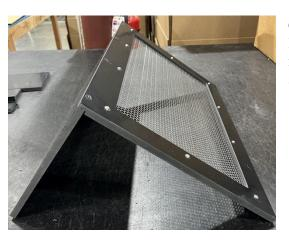
6. It is now time to assemble the internal hood. Locate Panels #6 and #7 and screw them together as shown. It is important to make sure that the rear of these parts are aligned as show.
