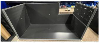
3. After Panels #2 and 3 are securely fastened, add the back face to the assembly, which is marked as Panel #4. Before proceeding, make
