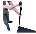
Please note: the connectors are designed to be tight and will usually require several firm hits with a rubber mallet to fully move into place. It's quite normal to shave off some plastic on the connectors as they are hammered into place.
