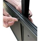
bolt. Hold the nut in position with either your pliers or an adjustable wrench and tighten the bolt using your screwdriver.
