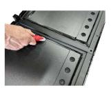
11. The front frame that you completed in step 1 is now ready to be seated onto the finished frame (Top, Bottom, Sides and Back) but before you do, now is the best time to make sure the gaskets are firmly in place, on this part. We find this easier when against a hard surface like a floor and while it takes a little effort to press the gasket into the gap, it will help secure the panels in place and also help stop substrate from
