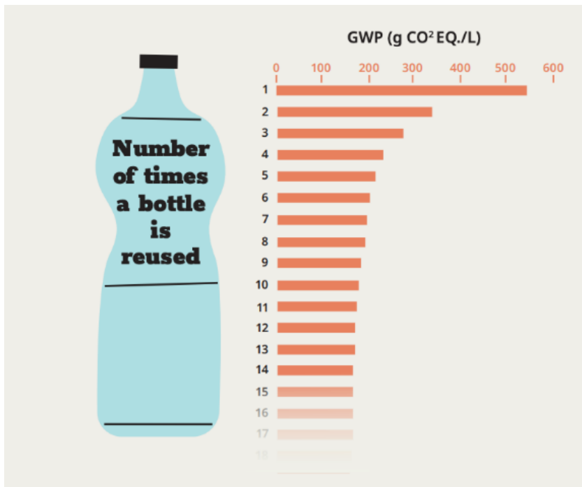
Number of times a glass bottle is reused and the decrease in Global Warming Potential g CE eq/l
