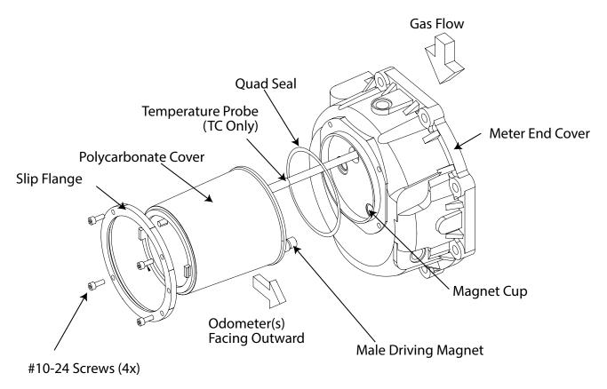
Figure 17 - Assembling Series 3 Accessory to meter end cover
