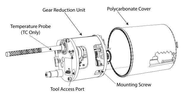
Figure 18 - Exploded view of Gear Reduction Assembly and Polycarbonate Cover
