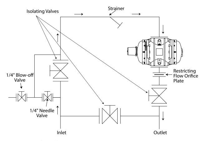
Figure 11 - Top Inlet Configuration for Series B3 Meter.
