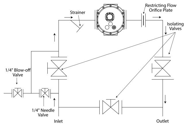
Figure 12 - Side Inlet Configuration for Series B3 Meter.
