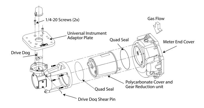
Figure 20 - Assembly Instrument Drive to meter end cover
