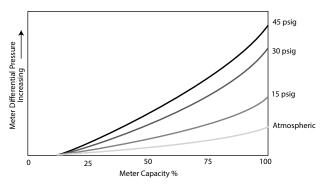
Figure 22 - Differential Curves change as pressure increases.
