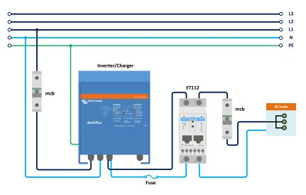
AC Meter - Wiring when used to measure AC output of an Inverter/Charger
