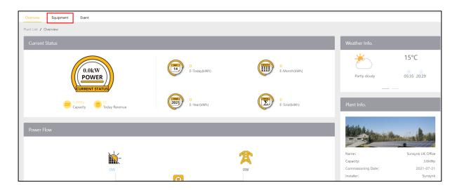
4) In the Equipment page, click the more button '(...)' in the upper right corner to set an alias for the device, perform remote upgrade, and change inverter settings / parameters, as shown in the figure below.
