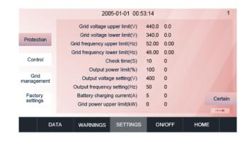
Grid voltage upper limit: If it exceeds Max. power grid voltage, it will switch to off grid mode. The default setting is 110% of rated voltage.
