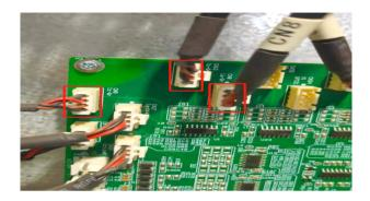
3. There are also corresponding number on the sampling cables (CN8, CN9, CN10, Grid-A, Grid-B, Grid-C)
