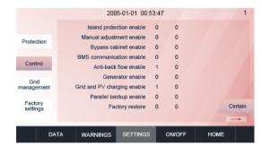
Island protection enable: it is a protection to prevent the inverter from not correctly switching into off grid mode in case of grid abnormality. Enter 0-9,0 means disable; 1-9 means level, suggested not to set too high.
