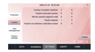
Number of parallel machine: number setting of parallel system. When 2 inverters in parallel, set as 2; when three units set as 3.
