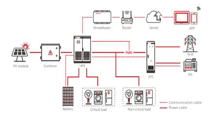
5. The direction of the arrow on the Halls should be towards the grid side.
