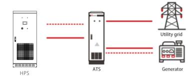
3. There are three circuit breakers in ATS. The middle circuit breaker is connected to the power grid switch (AC input) of HPS. The other two are grid switch (grid) and generator (Gen) switch. Pay attention to the printing on cabinet. It is not allowed to connect incorrectly, neither is it for the three phase sequence, otherwise the system cannot operate normally.
