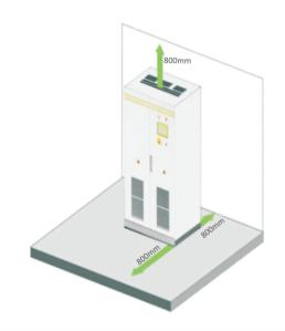
In front of the installation place of inverter, a space of 0.8m or more shall be ensured, the back 0.8m or more, the top 0.8m or more to ensure easy installation, cooling and maintenance.
