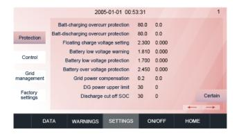
> This page is the battery parameter setting page. As battery is an important part of the energy storage system, the battery parameters need to be carefully confirmed whether they are consistent with the actual situation.
