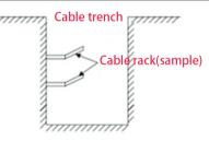
The cable trenches are often designed and constructed by the construction side based on relevant standards, with the equipment weight and dimensions required to be considered. Good electrical connection is needed between different cable trenches and GND terminals.
