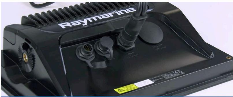
**Step 1: Connect the RayNet adaptor cable into display.**
