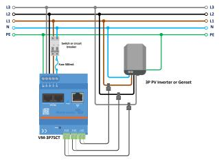
VM-3P75CT 3 Phase Wiring - Role is set to measure a PV Inverter (or Generator)
