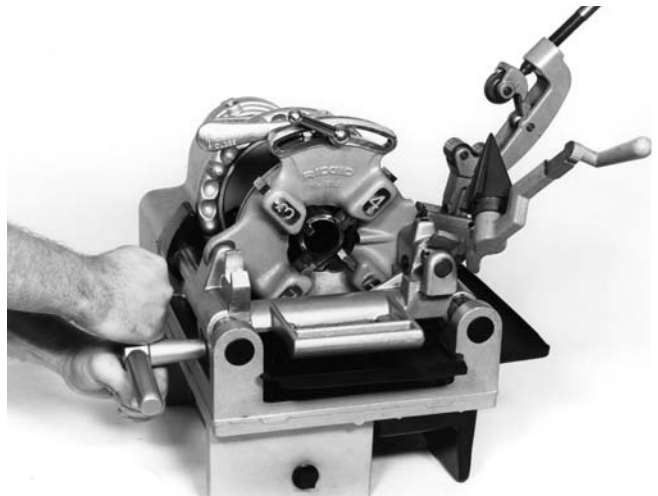
Figure 7 – Threading Pipe With No. 811-A Die Head
