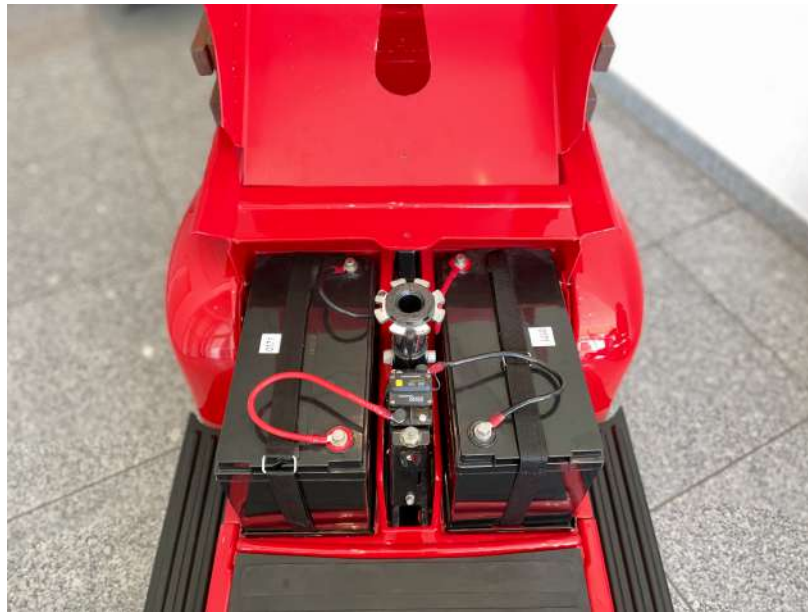
Figure 7: Batteries and battery connections
