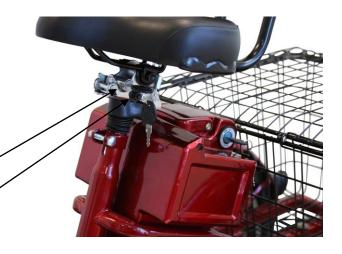
Key Lock - Stabilizing Bolt
