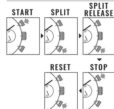
Measurement and release of split time can be repeated as many times as necessary by pressing the button **B**.
