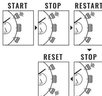
Restart and stop of the stopwatch can be repeated by pressing the button **A**.
