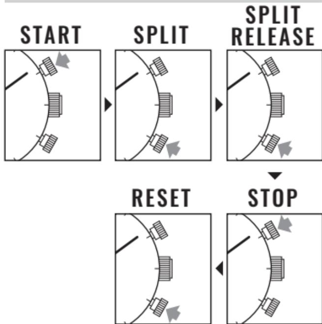
Measurement and release of split time can be repeated as many times as necessary by pressing the button **B**.
