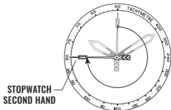
The approximate average speed within the distance can be determined by observing the present position of the second hand and reading the outer bezel.
