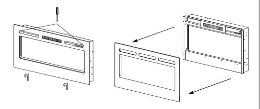
Remove 2 x screws that secure the wall bracket to the fire. Then remove the 2 x screws that secure the fixing plate to the fire.
