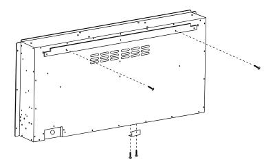
Mark the holes required for the wall bracket. Ensure these holes are level and drill 6mm diameter holes approximately 35mm deep. Insert the wall plugs and screw the wall bracket to the wall.
