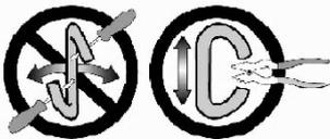
**Notice: It is important to use proper chain pliers (not included) To OPEN and CLOSE the chain included with this fixture. Do not open them with other tools that may twist or stress the chain links. It is important to use proper chain pliers like the ones shown in the diagram.**
