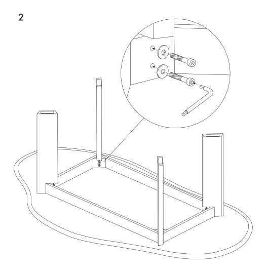
Screw two washers and two screws M8 into each table leg. Tighten with an allen key.
