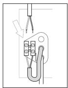
Connect the power supply cable to the connector block as shown in the diagram. Ensure that the connections are tight and that no loose strands of wire are sticking out from the connector block.
