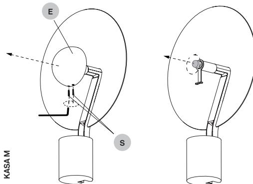
In order to change the bulb in KASA M, first remove the semiespherical reflector (E) using an allen key to undo the screws (S). Then you will be able to access the bulb to change it.
