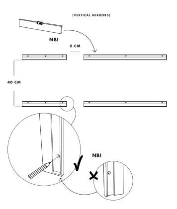
DRILL HOLES IN THE WALL AT THE POINTS THAT WERE MARKED IN THE PREVIOUS STEP 1. THE DRILL END IS NOT INCLUDED, WE RECOMMEND THAT YOU CHECK WHICH DRILL END IS SUITABLE FOR YOUR WALL.
