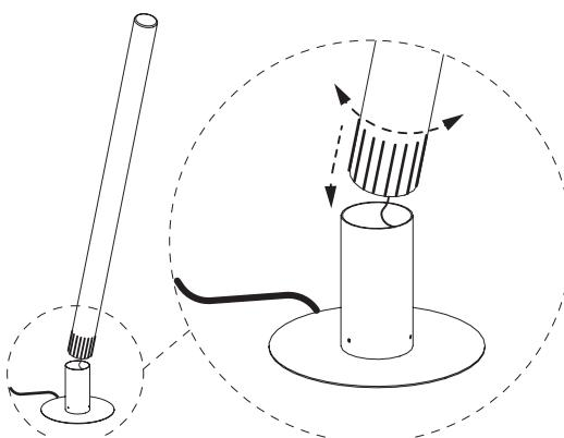
Once the connection has been made, carefully introduce the shade into the base tube.
