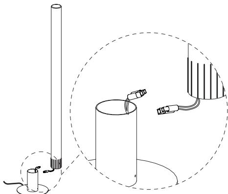
Connect the shade (A) to the base (B) using the quick connectors (C) attached to each part.
