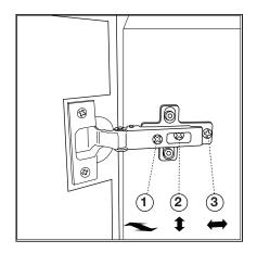
Use the **Phillips Screwdriver T1** supplied to adjust the door hinges:
